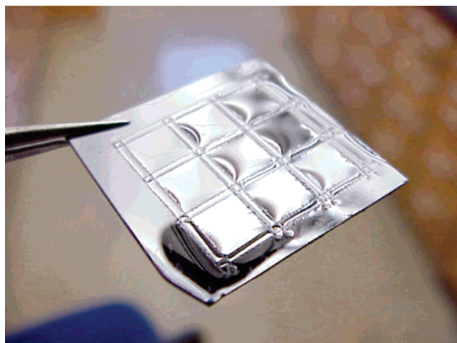
FIGURE 11. Hydrophilic silicon substrate containing hydrophobic lines after a rinse with DI water. Lab Chip 2004 , 4 , 553–557—Reproduced by permission of The Royal Society of Chemistry.
